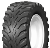
Tire for agriculture and green areas with rounded shoulder profile for small dumpers and mini loaders
